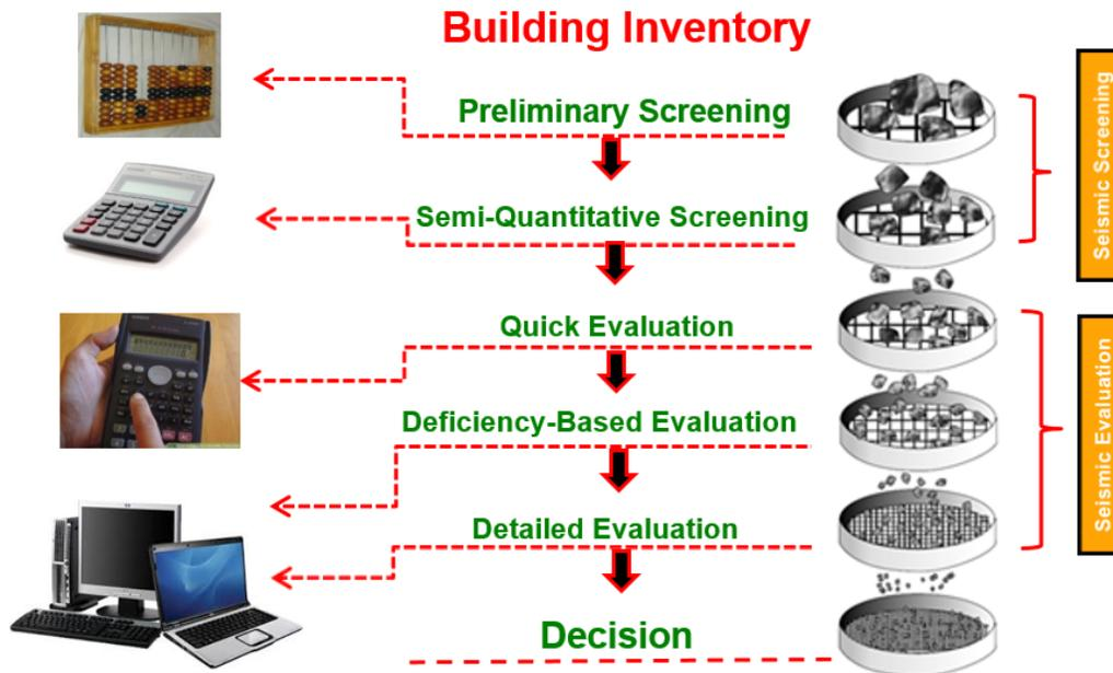
Figure 1. Components of framework for seismic risk management.
